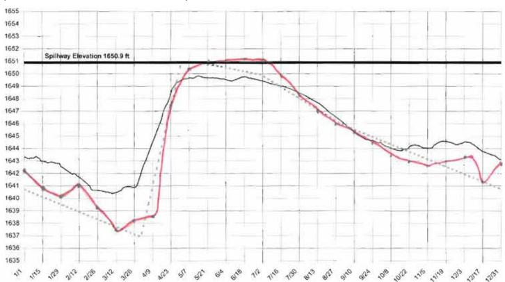
2013 ACTUAL ELEVATION - heavy line HISTORIC AVERAGE ELEVATION - thin line TARGET ELEVATION - dotted line
